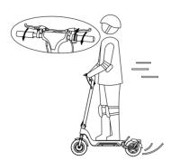
3. Put your other foot on the footrest to keep both feet stable. Press the throttle on the right handle to speed up once you are balanced.
