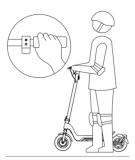
DO NOT press throttle when walking with the Electric scooter.
